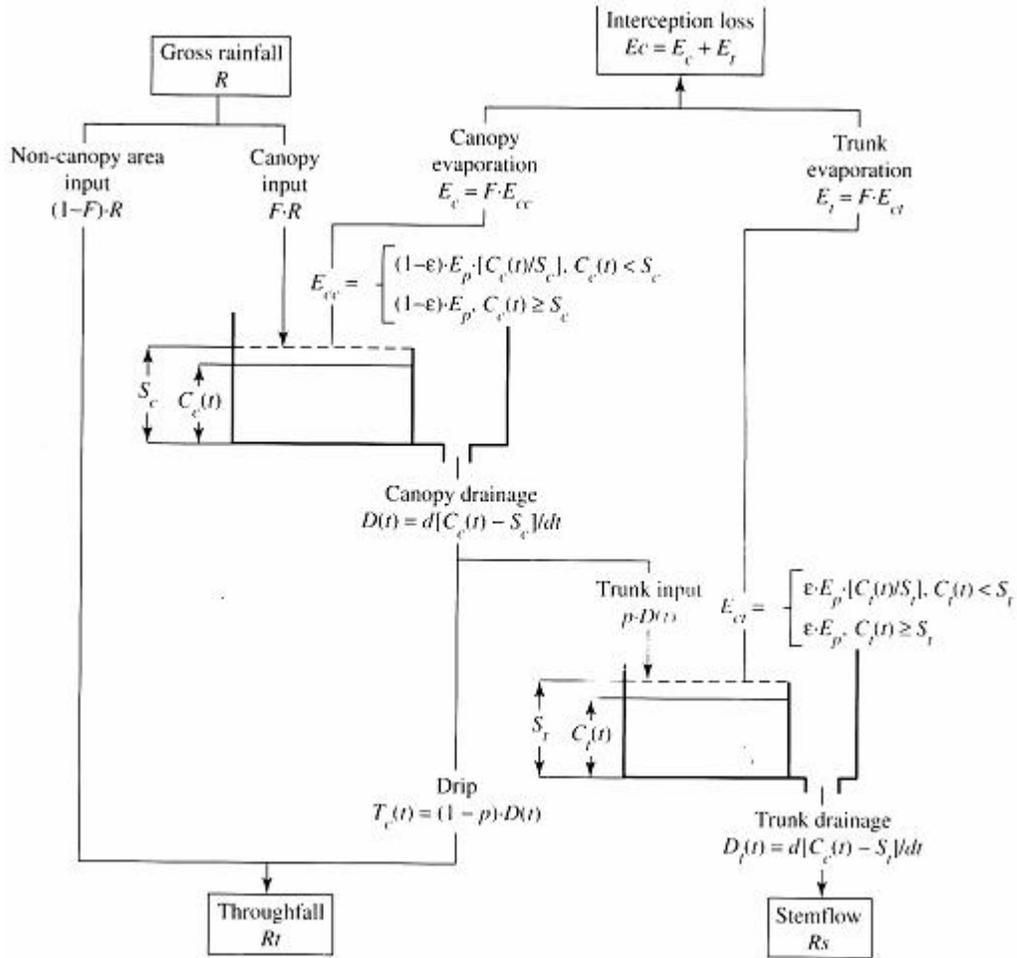
Figure 2. the schematic diagram proposed by Valente et al. (1997) for canopy interception loss (Dingman, 2002).
