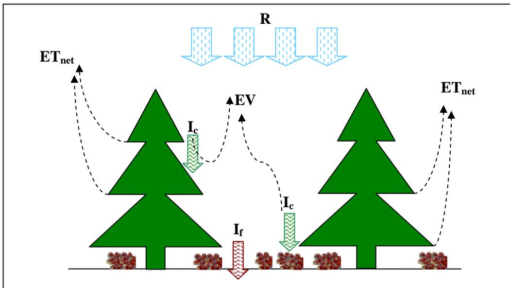
Figure 3. A schematic diagram of the simplified interception module in the MSDW model.
