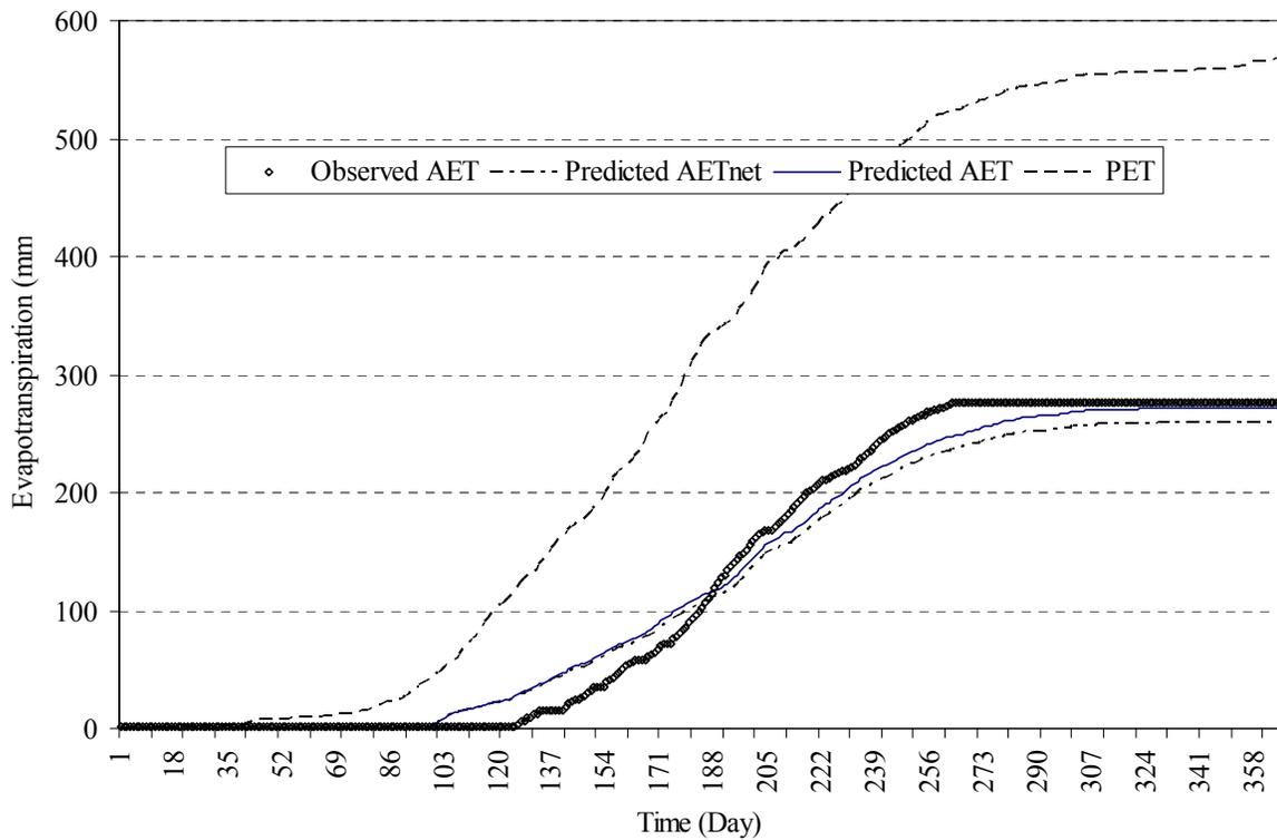
Figure 10. Observed and predicted Evapotranspiration (mm) in the SBH site.
