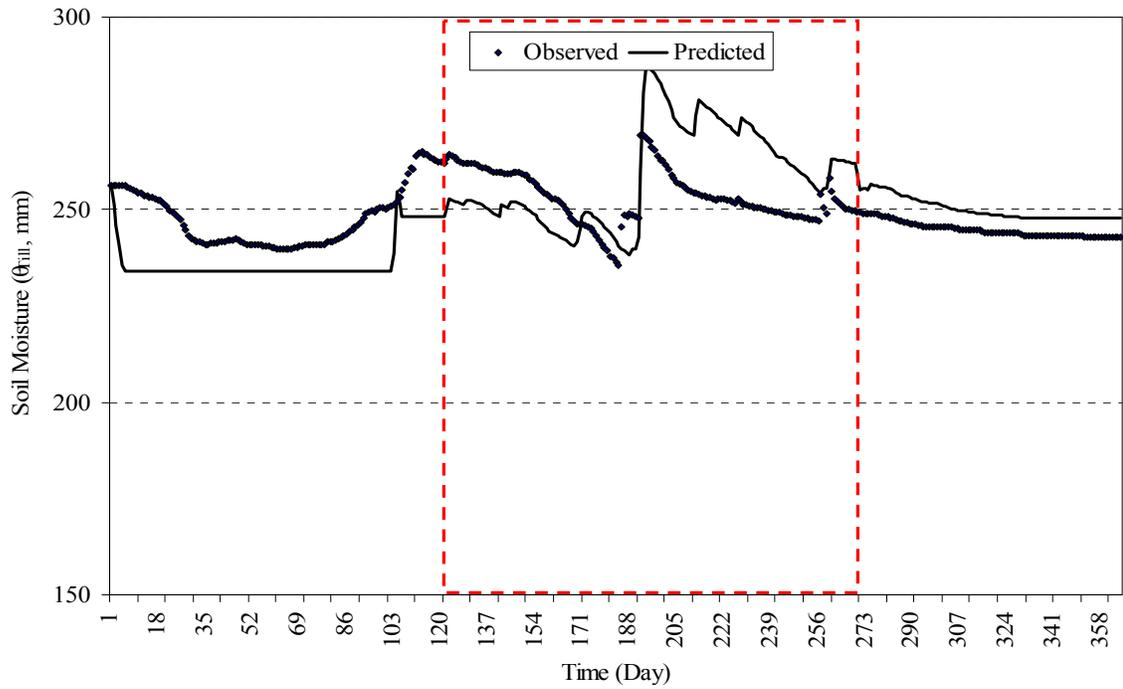
(b) Figure 9. Observed and predicted soil moisture content in the SBH site: (a) upper layer (peat); (b) lower layer (till)
