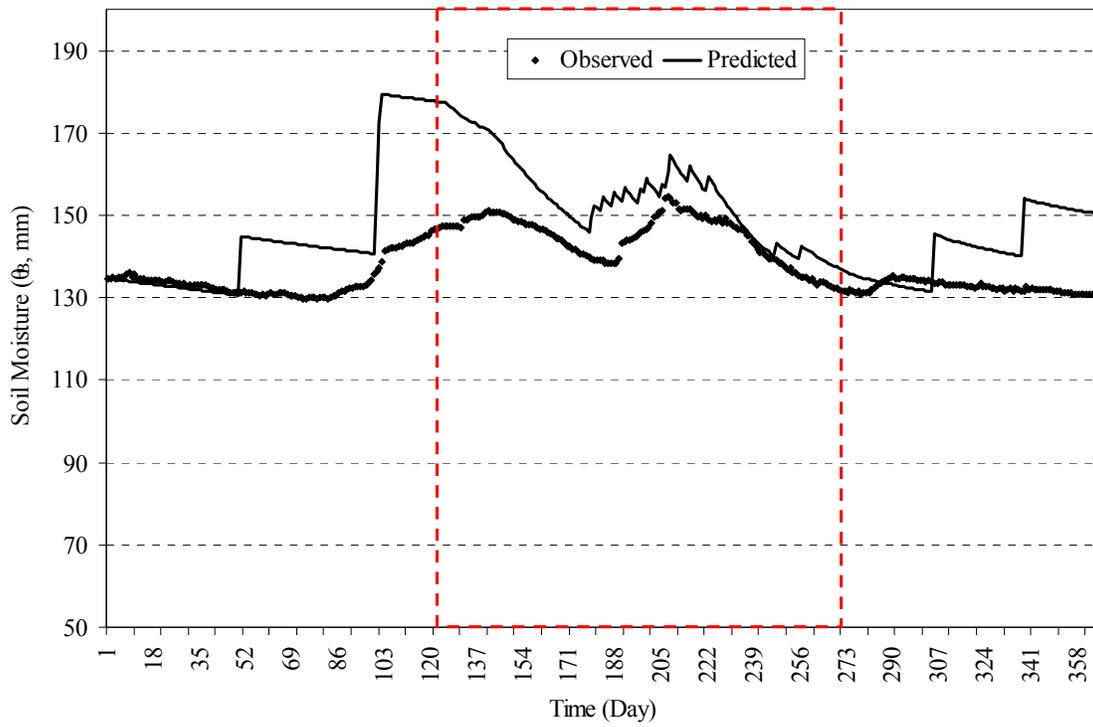
(b) Figure 11. Observed and predicted soil moisture content in the Old aspen natural site: (a) A-horizon; (b) B-horizon.
